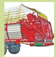
A uniformly distributed blanket of forage is essential for perfect compression. The discharge system features three beaters to protect the machine and make life easier for the driver. A twobeater system is also available for working in clamps.
