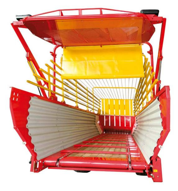
Opening the tailgate conveniently from the driver's seat is a standard feature. The full crosssection of the tailgate is open to allow rapid and unrestricted unloading.
