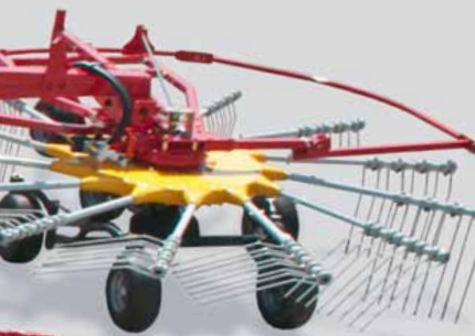
Retract one of the front rotors to circumnavigate obstruction
