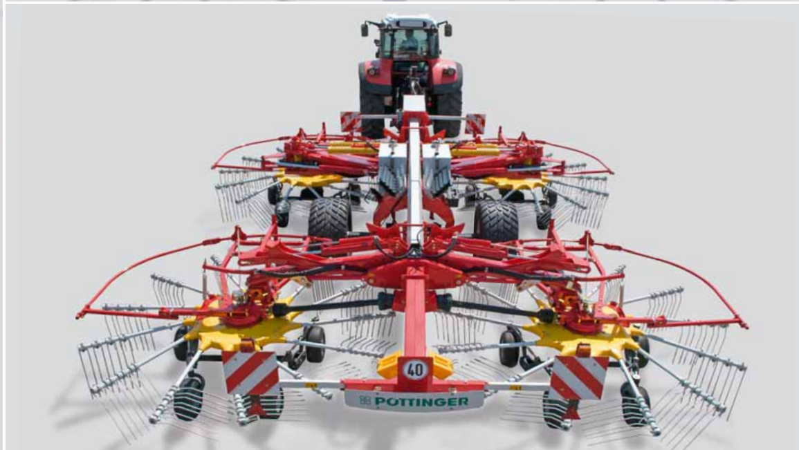
Retract one of the front rotors to circumnavigate obstruction
