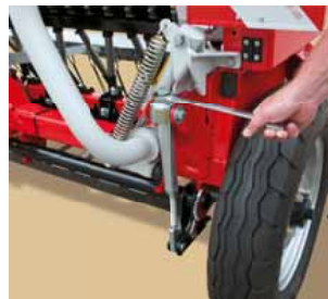
Central coulter pressure adjustment
