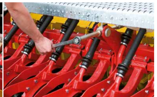
Central coulters pressure adjustment
