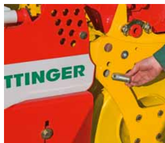
Remove fixing pins on rear roller for Parallelogram guidance
